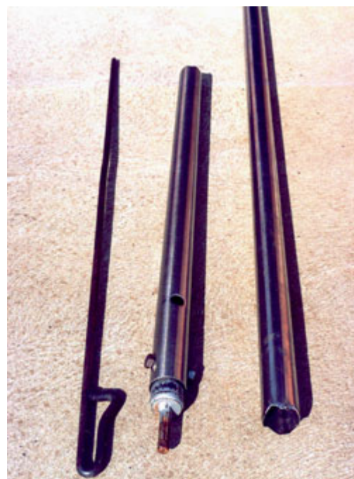
Figure 1. Simple corer made from stainless steel tubing
